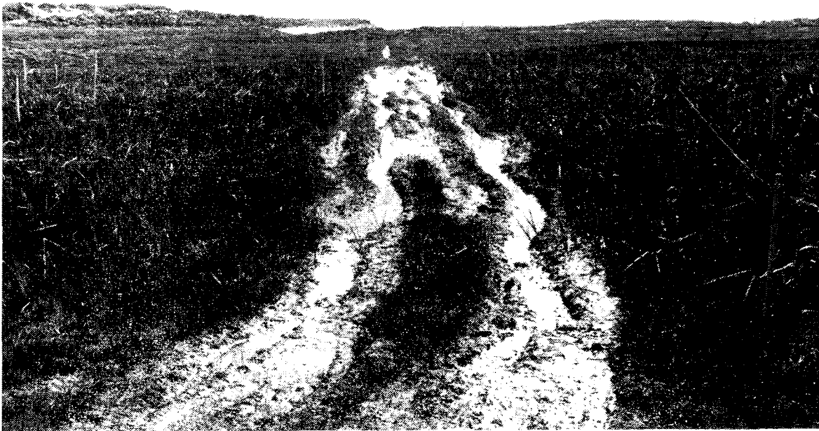
Fig. 13. The low marsh ( Spartina alterniflora ) was reduced to a quagmire and became impassable after only 90 passes.
