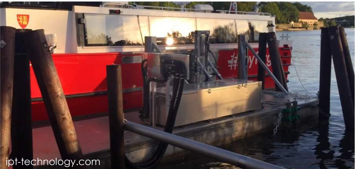
Figure 13: Double ended, roll-on-roll-off vessel (above). IPT Technology wireless, on-shore inductive charging system (bottom).
