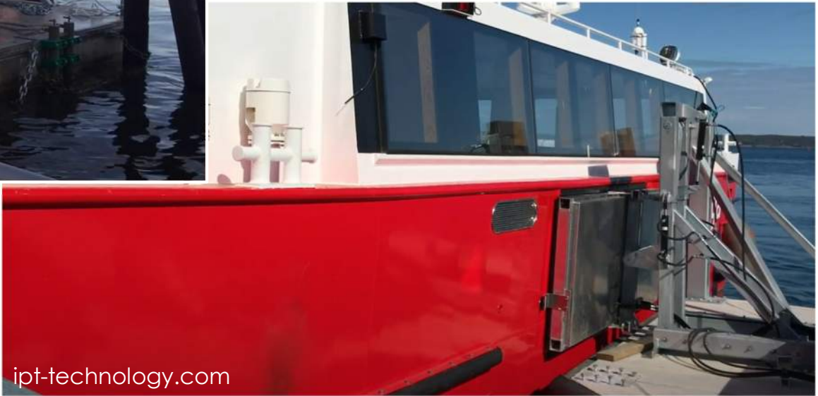
Figure 13: Double ended, roll-on-roll-off vessel (above). IPT Technology wireless, on-shore inductive charging system (bottom).
