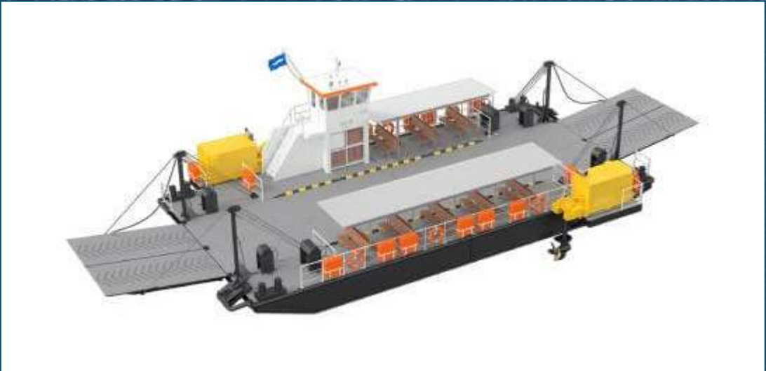
Figure 12: Example of proposed small double-ended ferry vessel equipped with deployable ramps. Photo and ferry design by Damen.
