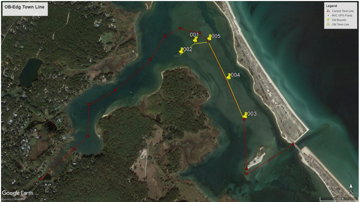
Map of the Edgartown-Oak Bluffs town boundary in Sengekontacket Pond. The yellow thumbtacks represent the location of the concrete bounds. The red points represent the town boundary provided by the MVC (data source = MassDOT). Map produced using GoogleEarth software.
