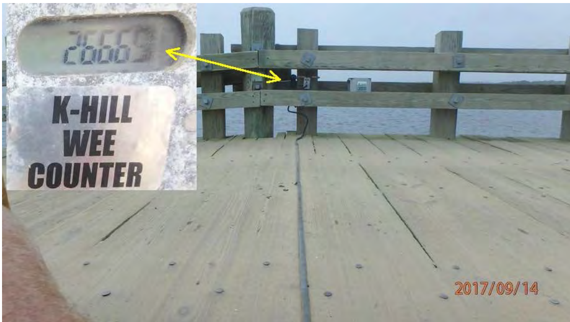
Photo 6: Midspan south rail, active traffic counter.
